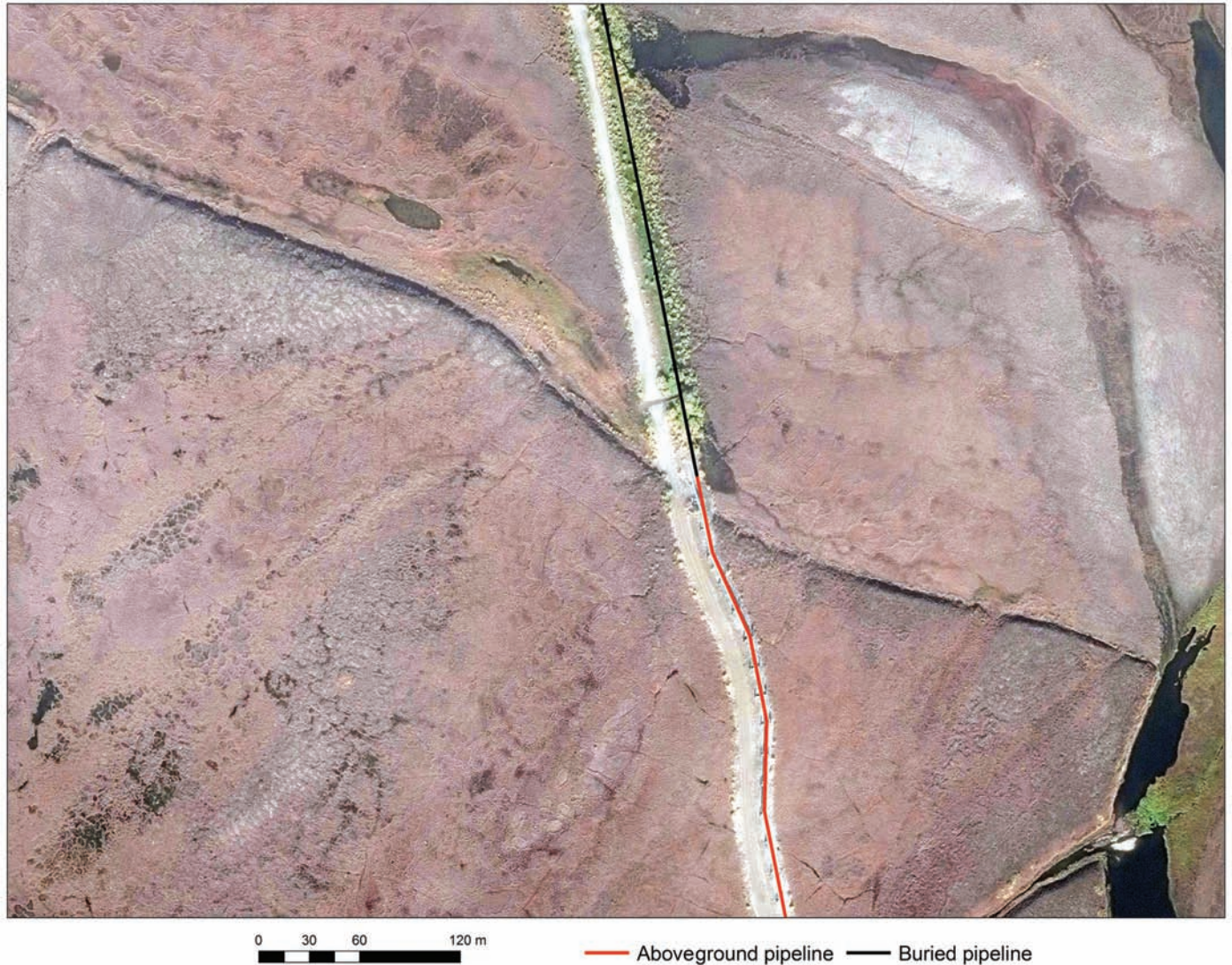
FIG. 5. Image from WorldView-3 (© 2016 Digital Globe, Inc.) showing the abrupt change in vegetation along the pipeline as it transitions from aboveground (red) to buried (black).
