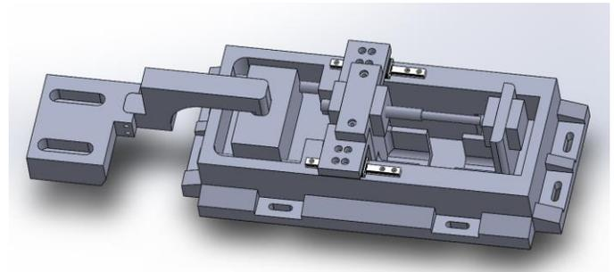
**Figure 1:** Final 3D model of loading device, with dimensions of approximately 280mm x 120mm x 110mm (length x width x height). The left side attaches to the linear actuator.
