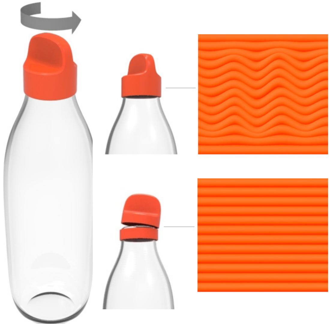
At left, potential benefits of corrugating Z-layers in an FDM 3d printed bottle cap design (for upcycling glass water bottles). At top right, corrugations would prevent twisting shear over parallel layer deposits shown at bottom right.
