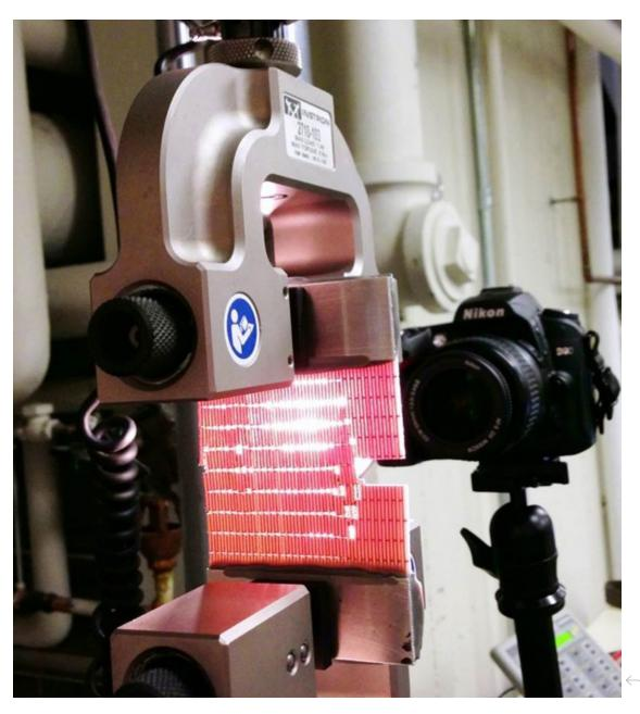
Experimental setup in which the 3D printed composite material is tested under extreme mechanical loading. This setup is used to extract strength and toughness and other mechanical properties of the material.
